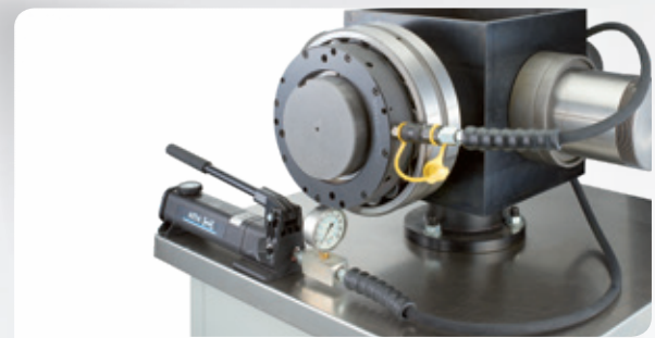
Mounting on sleeve with a hydraulic nut
