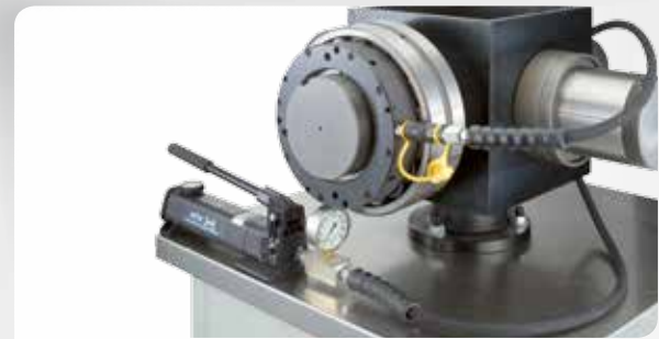
Mounting on sleeve with a hydraulic nut
