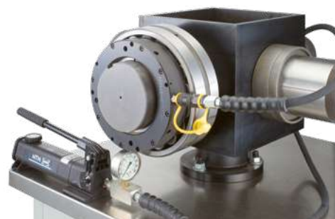
Extraction of the withdrawal sleeve with a hydraulic nut
