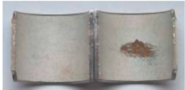
Fig. 35: Local damage caused by cavitation
