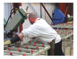
Alwayse **FLOAT-ON** castors have been specifically developed for use in wet and dry conditions. Available in; Bright Zinc Plate (BZP) which is suitable for most applications, and Stainless Steel INOX (S/S) for use in the most arduous of conditions.
